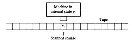
We assume that the machine must be in internal state  $q_0$  to commence operating. The machine operates in discrete steps, its action at any stage being determined by its internal state  $q_i$  together with the symbol  $s_j$  printed on the square being scanned. The possible actions of the machine are of the following kinds:
